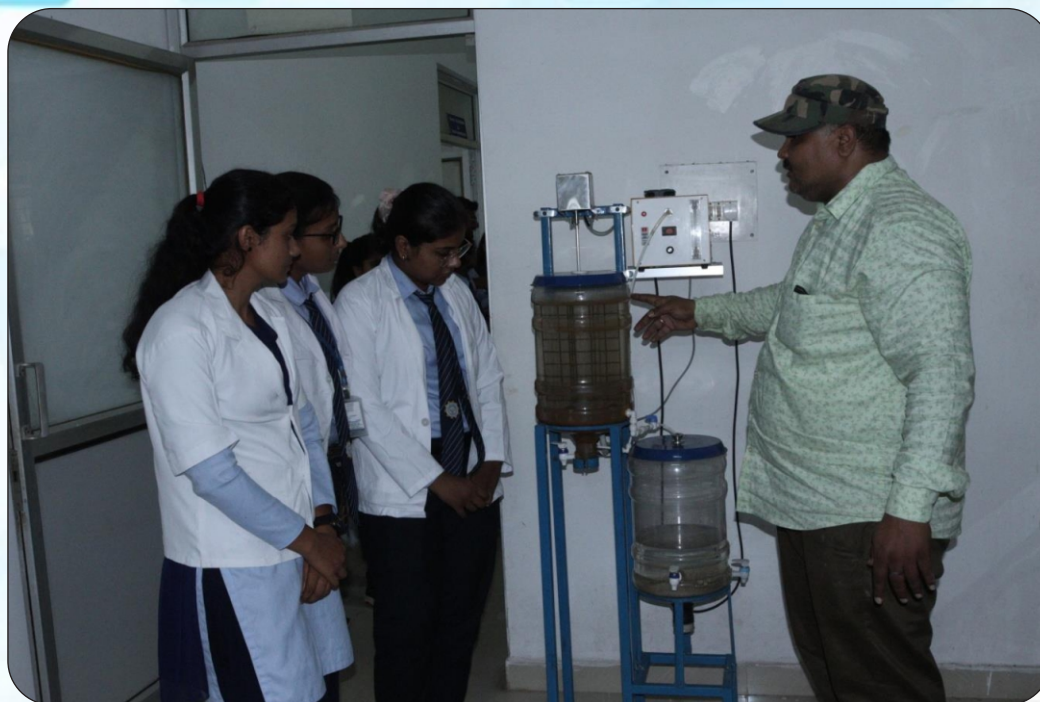
Figure 3: Assembly for Arsenic Removal
