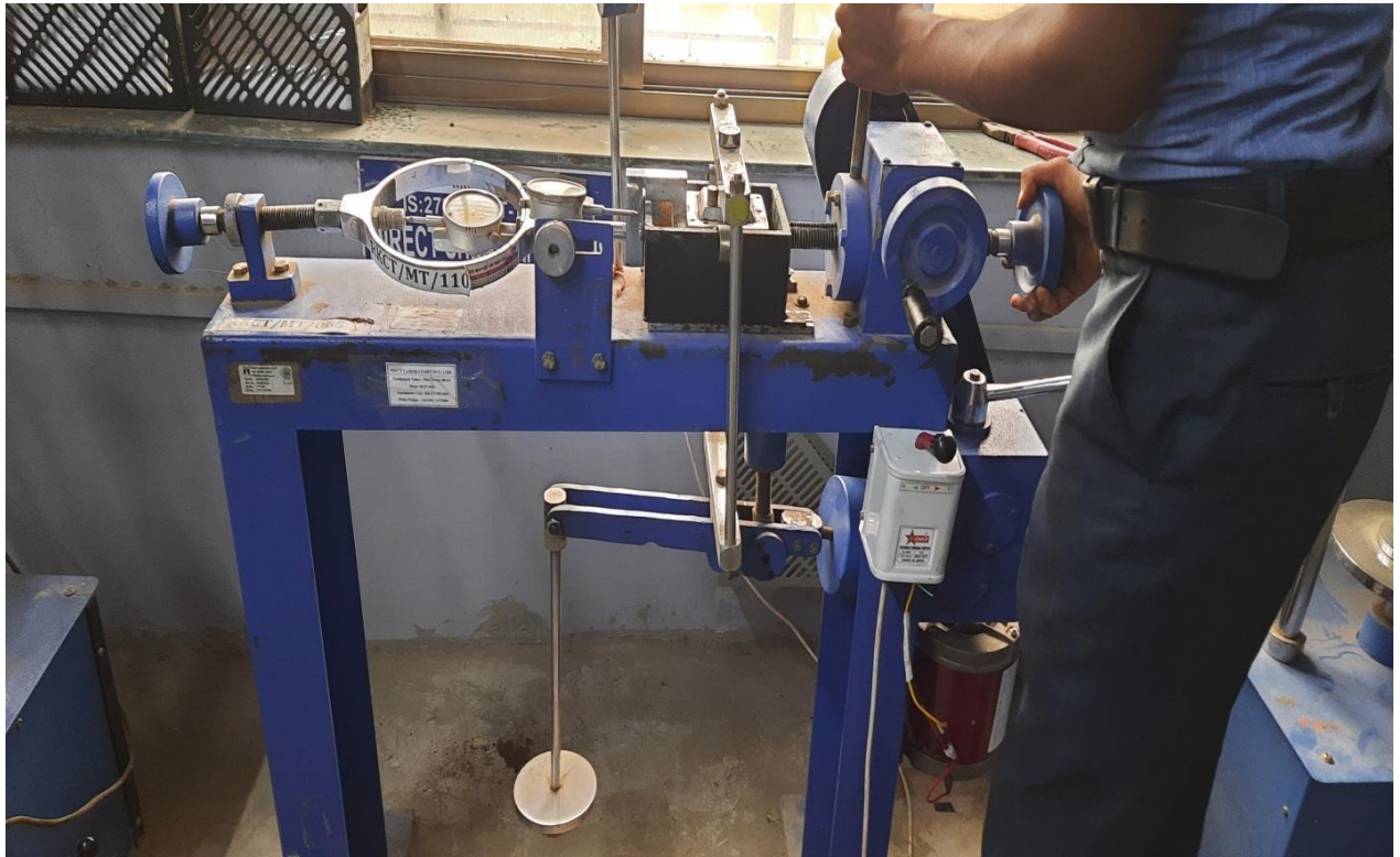
Photograph 7 Direct Shear test of sample at RKCT laboratory, Jabalpur
